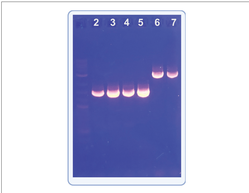
Figure 2 Gel electrophoresis visualization of colony PCR results to validate the presence and modifications of a mutant. Primers flanking each side of the aceE gene-deletion site were used, yielding products of \sim 1.5 kb for successful mutants and \sim 2.8 kb for wild-type strains. From left to right: lanes 2-5 display successful aceE gene replacement with the antibiotic cassette, lane 6 represents an unsuccessful attempt, and lane 7 serves as the wild-type KPPR1 control.
